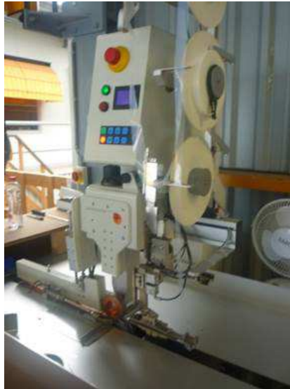
Ultrasonic head of a Jentschmann Weldsonic machine 2796-2-20
